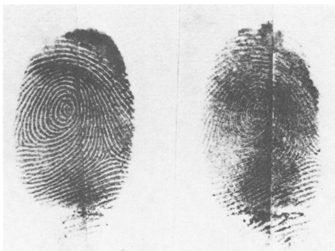
FIG. 4—Right half of each print "scrubbed" vigorously with an MeOH-saturated swab after prints deposited. Left half is the control. Ninhydrin development followed swabbing.
